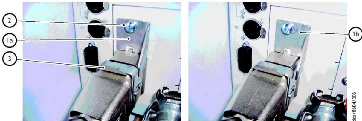
Figure 6 - Electrical connector locking mechanism
