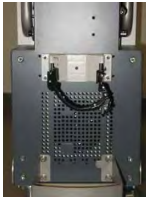
Bottle holder fixed on the leak detector
