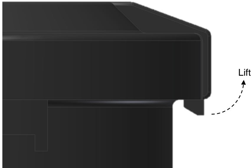
Figure C.2.1: Housing tab release.
