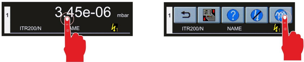
Fig. 29 – Switching the degas function On
