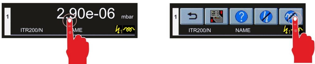
Fig. 30 – Switching the degas function Off
