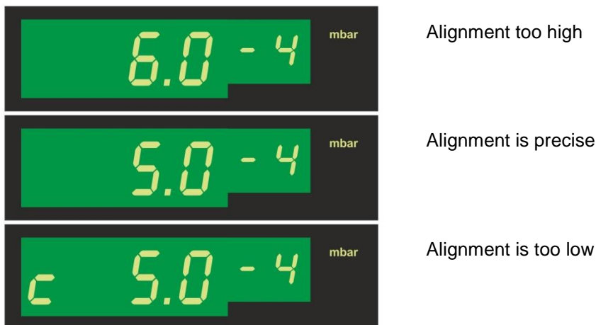
Figure 18 – Zero alignment for the THERMOVAC gauge head
