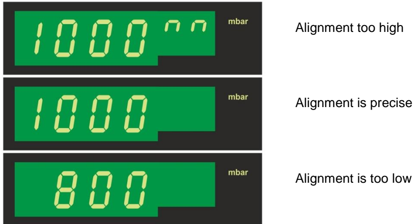
Figure 17 – Full-scale alignment for the THERMOVAC gauge head
