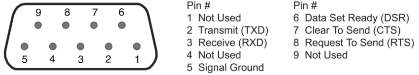
Figure 2-11 I/O (RS-232) 9-Pin Connector (pins)
