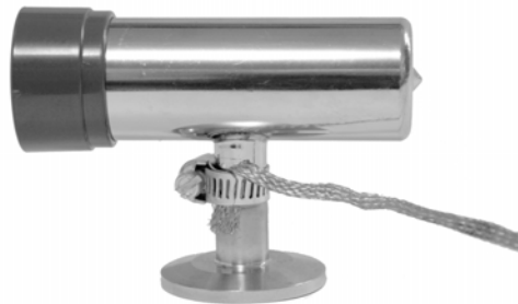
Figure 2-8 Convectron Gauge to Vacuum Chamber Ground Connection
