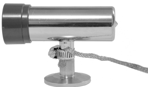
Figure 2-8 Grounding a Convectron Gauge
