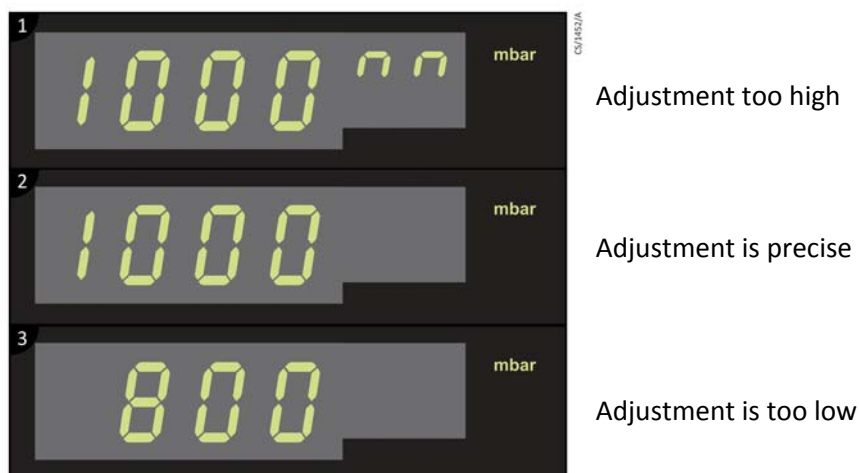
Figure 12 Full-scale adjustment for the PRG gauge head
