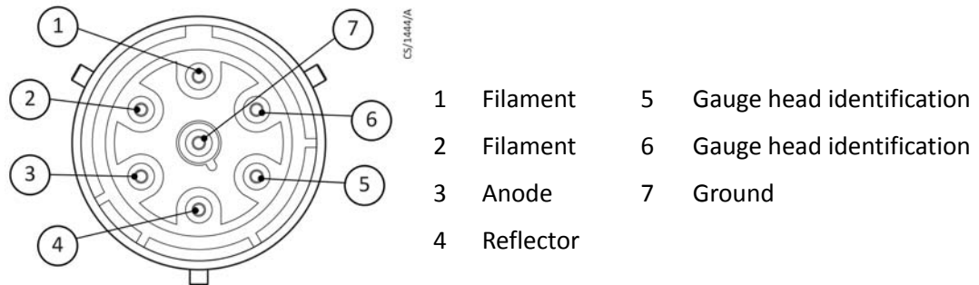
Figure 6 Connection for the IG gauge head (Metalock Bantam UTG0187SVDEU)
