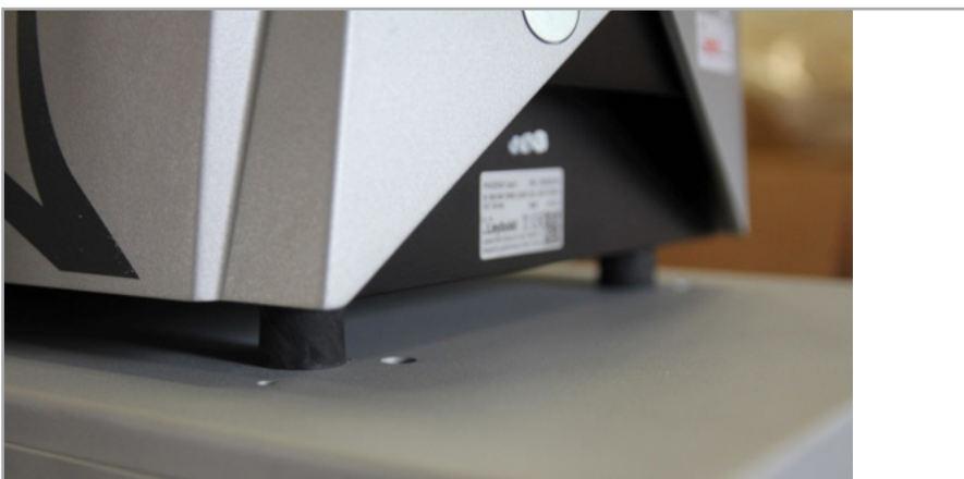
Fig. 4 Mount the leak detector with the rubber feet
