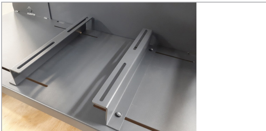
Fig. 6 Z-rails fixed to the cart
