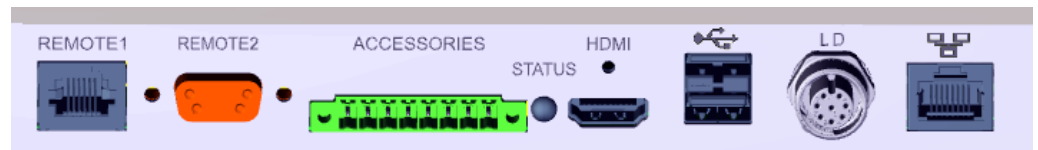
Fig. 5: Connections for accessories and control signals at the back side of the device.
